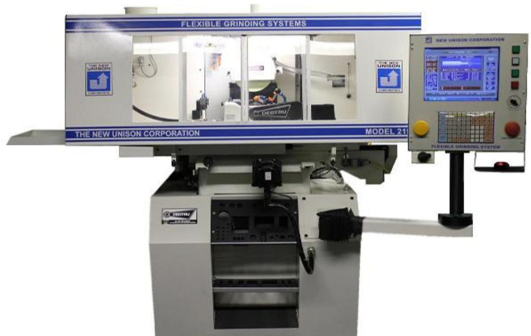
Unison manufactures nine versions of its Flexible Grinding System (FGS). Each of these machines use Unison's proprietary software and motion control. The FGS Series is constructed on a cast iron base which has been hand scraped to insure the highest level of accuracy. Precision ground ballscrews are installed to provide smooth motion control and increase both the accuracy and longevity of the FGS Series machines.
